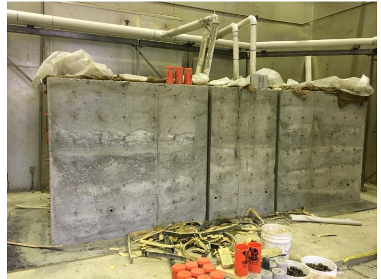
NIST Alkali Silica Reaction Test Setup
